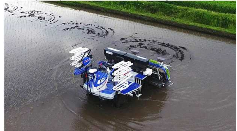
Autonomous unmanned vehicle for rice-planting (Autonomous demonstration in the test field)
